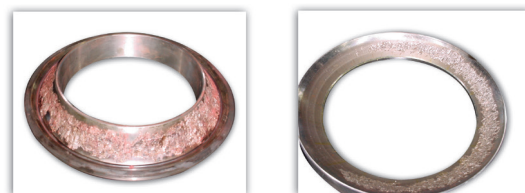
Circulating Water Pump bearing/race as found after APR notification of abnormal conditions
