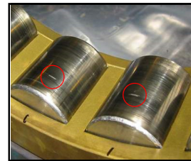
Wear marks on bearing
