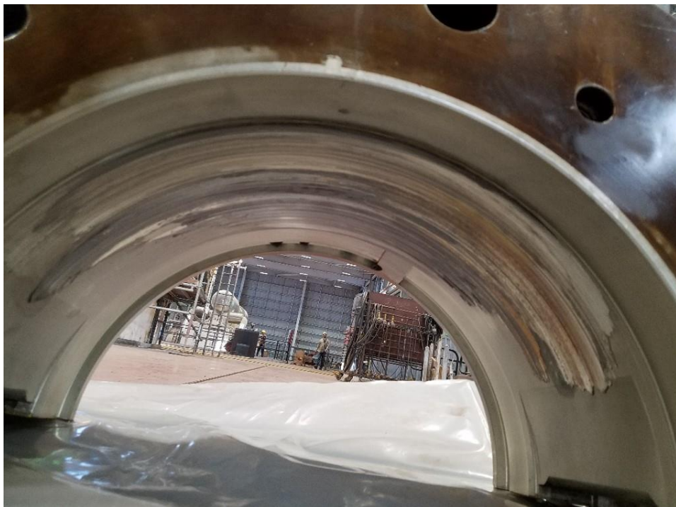
Damage found on steam turbine journal bearing. Conditions indicate rub occurred.
